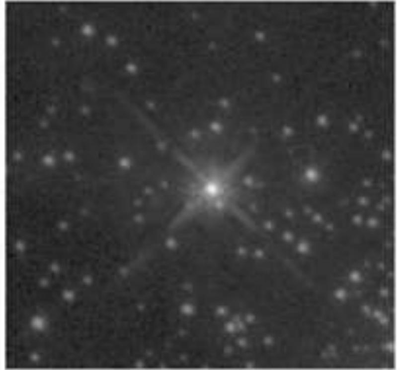
Due to an oversight during fabrication, the concave shape of Hubble's primary mirror was too shallow toward its outer edges by 2 microns, a tiny fraction of the width of a human hair. As a result, starlight was not brought to a focus at the same point, resulting in blurry images. These three images show the same star as viewed from a ground-based telescope, left, and from Hubble's uncorrected mirror, center. The corrected image, after a space shuttle repair mission in 1993, is seen on the right.
